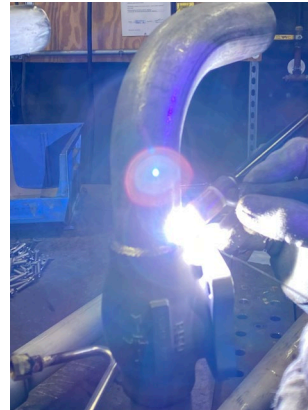
TIG Welding SKL9412SW (Stainless Steel Globe Valve)
