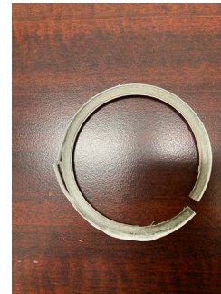
Over Torqued Body Gasket
