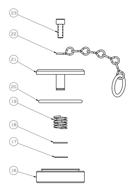
Figure 2 – Exploded Cap Assembly
