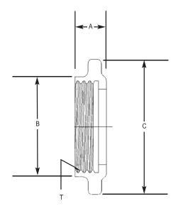
Material - Cast High Standard Magnesium Bronze per ASTM B584
