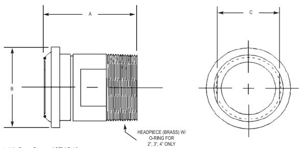
Material - Brass Bar per ASTM B-16
