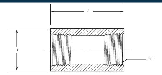
Material - Type 304 Stainless Steel per ASTM A276
