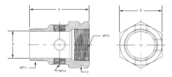
Material - Brass ASTM B16 shipped complete with two ½" Brass Pipe Plugs
