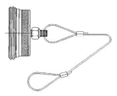
Material - Brass Bar per ASTM B16, with Stainless Steel Safety Cable
